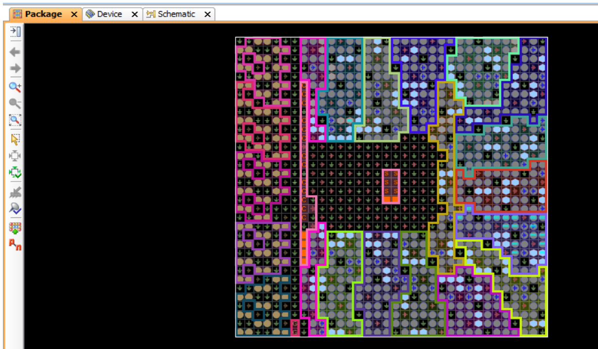
Figure 9. IO Planning of SubByte Transformation
